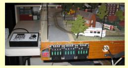
By October 16th, the Digitrax Zephyr was able to be connected to both Module 970, shown above, and the SCTC test track. Both are equipped with Innovator 3500 analog control systems and the track is electrically accessed via a DPDT switch that prevents DCC signals from entering the Innovator throttles.
